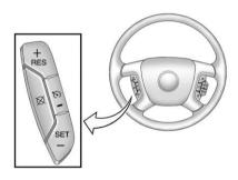
Press to turn cruise control on and off. The indicator comes on when cruise control is on.
